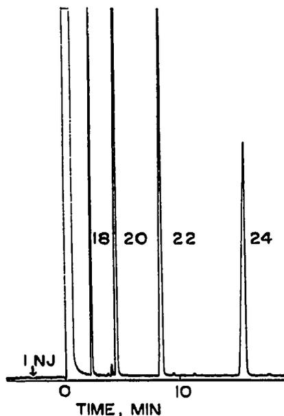
Fig. 1. Isothermal separation of *n*-alkanes with a 30 m × 0.3 mm I.D. glass capillary column (SE-30 phase) at 225°. The injection system permits the use of the usual type of solutions (1- to 5- $\mu$ l samples). The full-scale chart response usually corresponds to  $3 \times 10^{-11}$  A.
